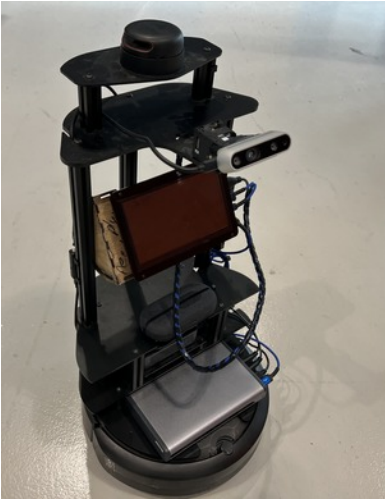
Figure 1: Hardware setup of the Socially Cognizant Robotic Campus Guide
